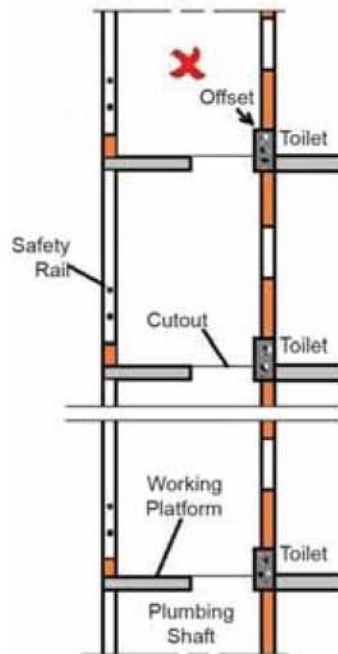
Figure 3.1.4: Structural Obstructions in Shaft-Section
