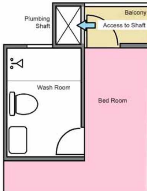
Figure 3.1.2b: Location of Shaft
