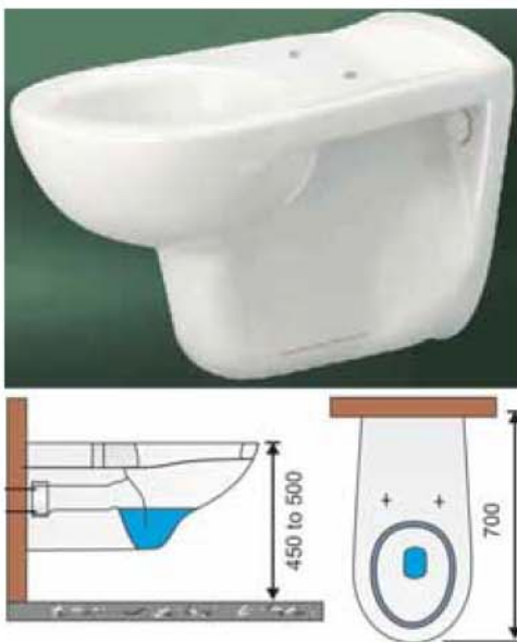
Figure 9.2d: Mounting Height of EWC
